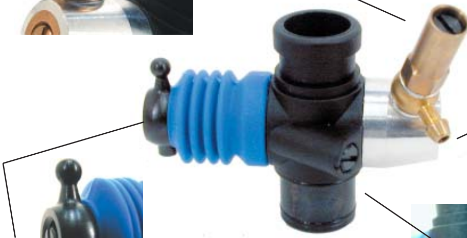
LOW END NEEDLE FACTORY SETTING: HEAD IS FLUSH WITH BALL COLLAR SET: 3.5 TURNS OUT FUNCTION: ADJUSTS THROTTLE RESPONSE.
