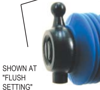
LOW END NEEDLE FACTORY SETTING: HEAD IS FLUSH WITH BALL COLLAR SET: 3.5 TURNS OUT FUNCTION: ADJUSTS THROTTLE RESPONSE.
